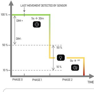
For more details on the operation and programming of the motion sensor see the **RC-HD05R USER GUIDE**  **Phase 0 :** As long as a person is detected by the sensor, the luminaire is at its maximum intensity. *Adjustable lighting level with* « Power % »
