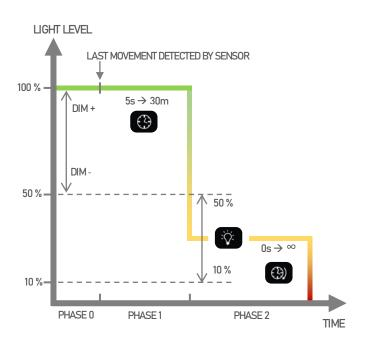
**Phase 0 :** As long as a person is detected by the sensor, the luminaire is at its maximum intensity.
